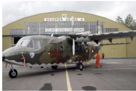
Figure 2. Propeller Hartzel HC-B4MN-5AL on CASA 212 Aircraft
